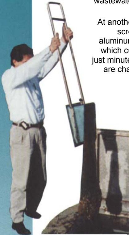
Removal of Dura-Sac Nosebox and Sack
